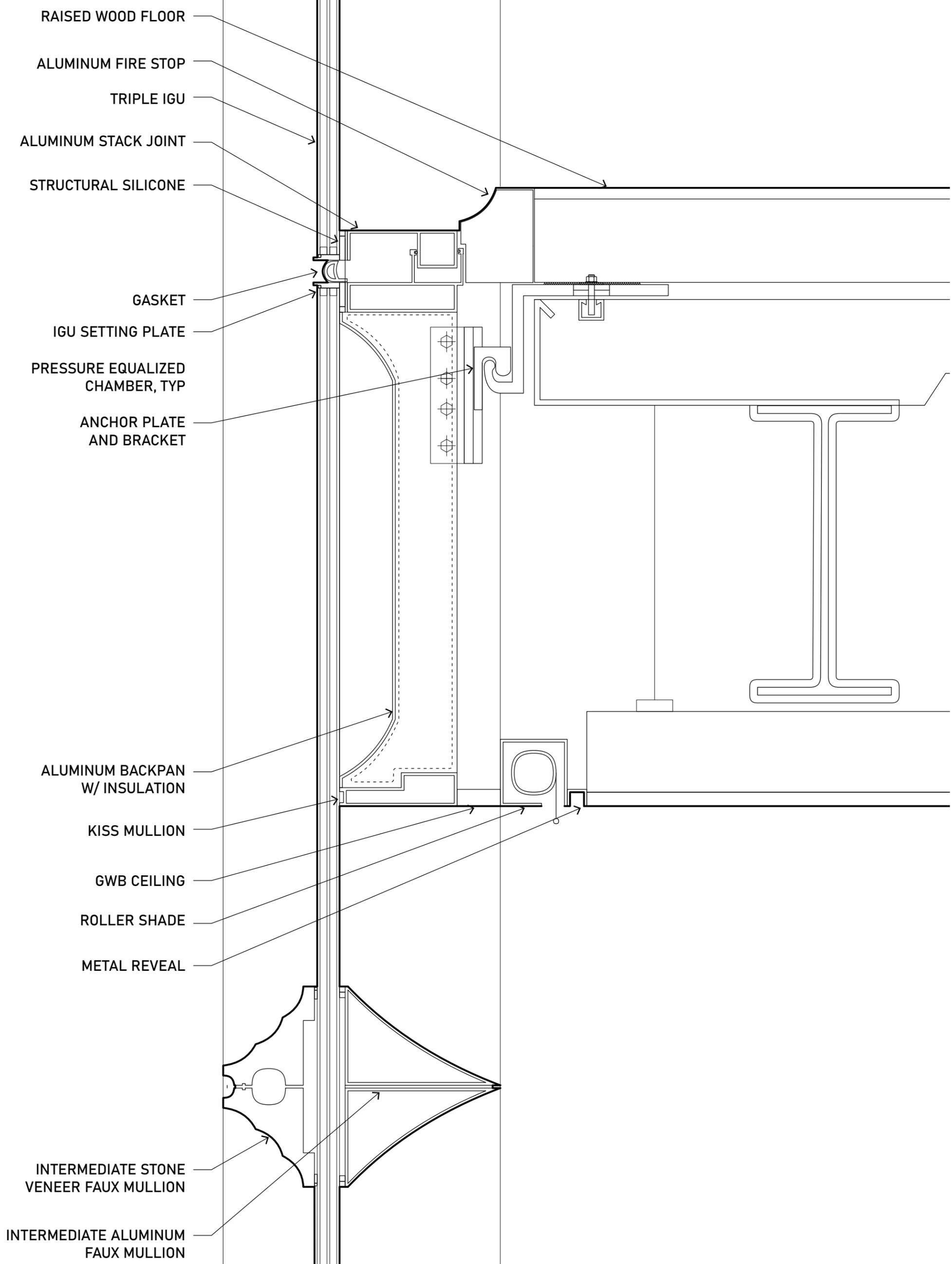
**B1** SECTION AT TYP. SPANDREL
