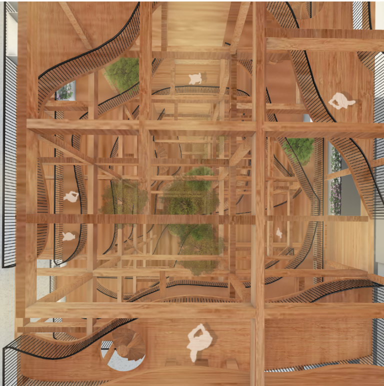
Balconies and voids through the core allow space for trees and plants to grow into the armature. Diagonal brace frames provide playful structural support in the interstitial space.
