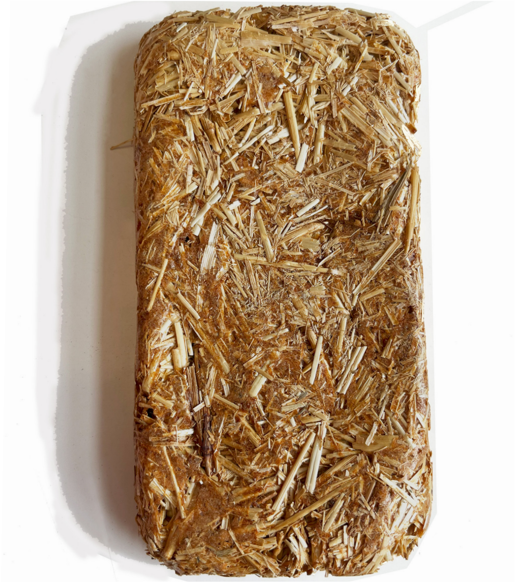
#01 Board: 1/2" compressed straw board baked with lime binder
