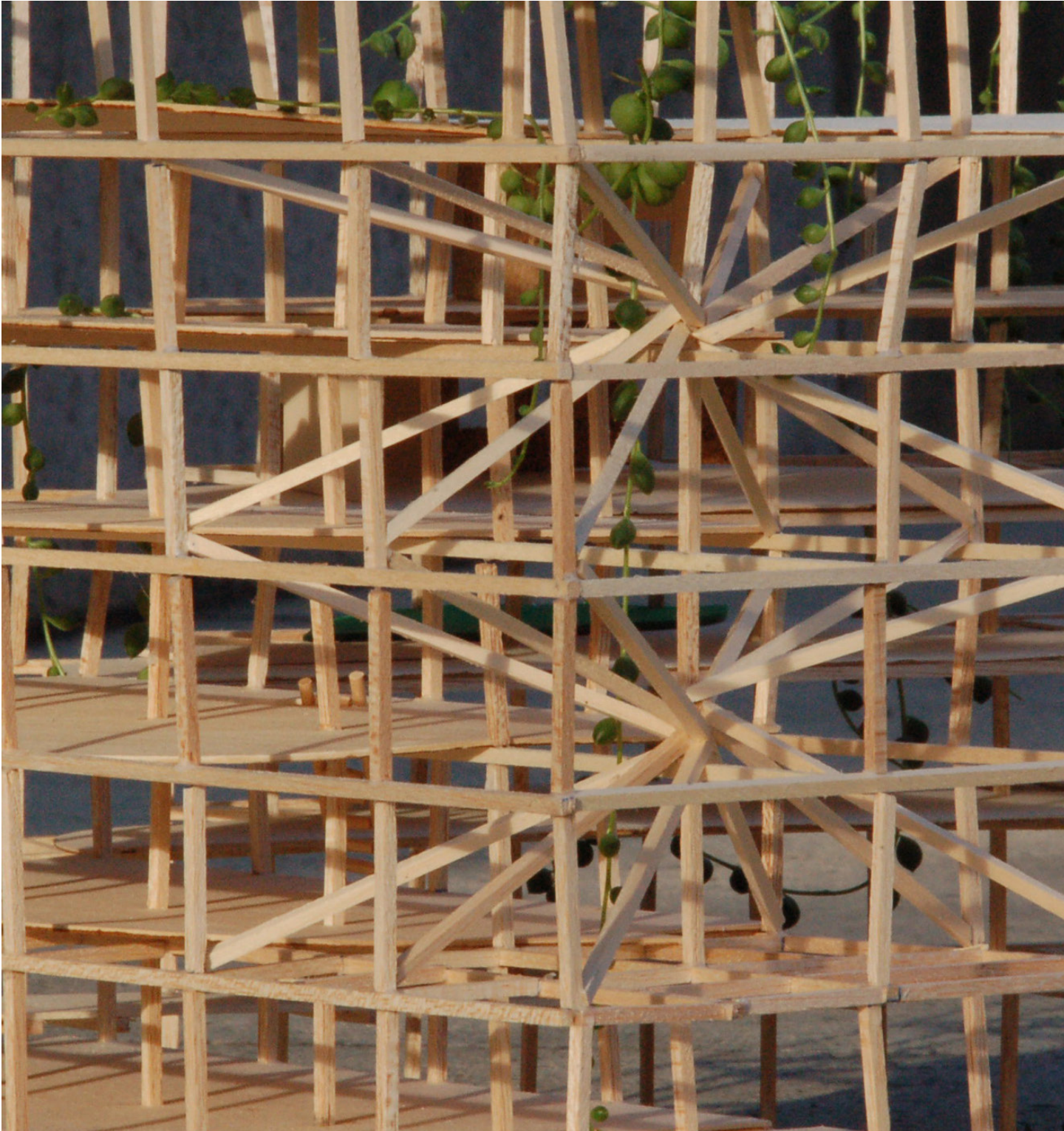
Brace frames through the central void provide structural support and opportunity for vines from the courtyard to grow.
