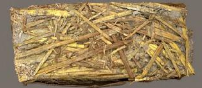
BIO-RESIN INFUSED RICE STRAW BRICK PRODUCED ON SITE
