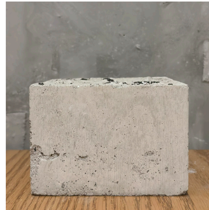
Asphalt Block Mixture : Cement+Sand+Asphalt aggregate + Water
