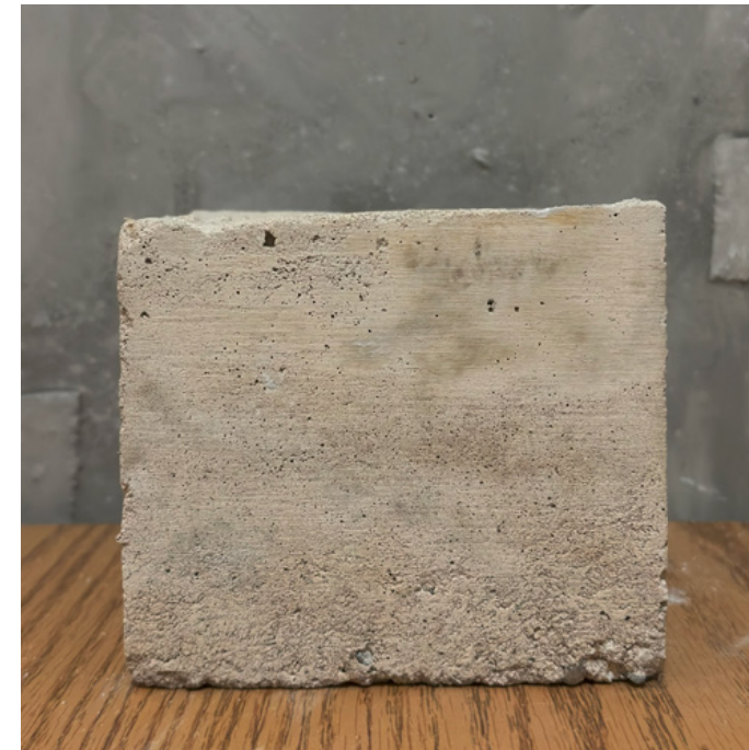
Traditional Concrete Block Mixture : Cement+Sand+Course aggregate + water
