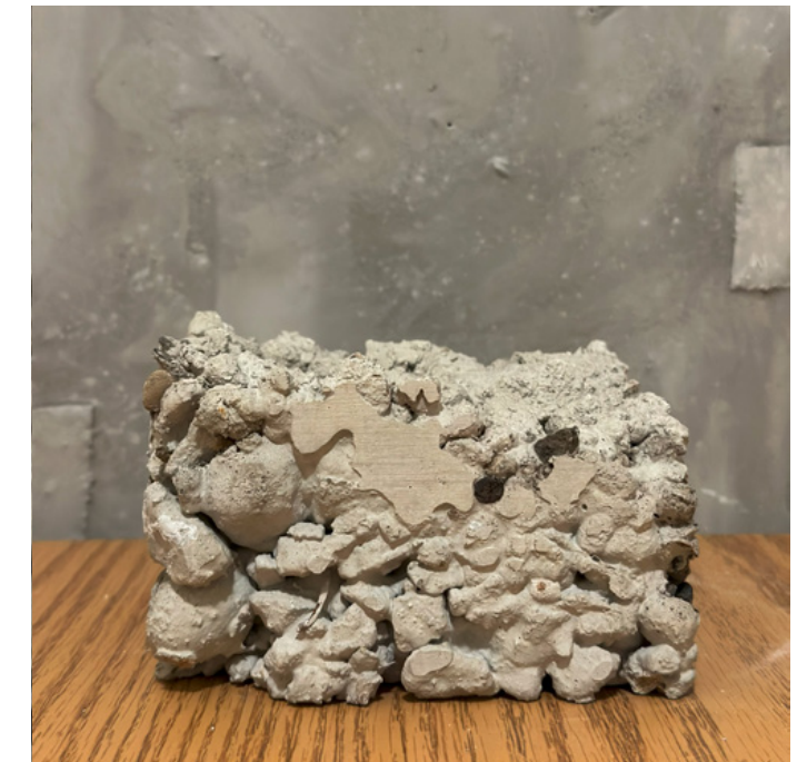
Porous Block Mixture : Cement +Asphalt aggregate + Water
