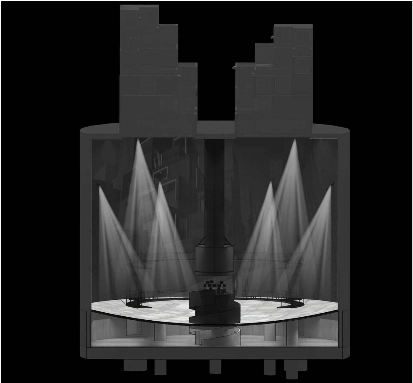
Drawing 1: A viewing machine built to optimize central orientation, with large windows and metal grating floors allowing the viewer to simultaneously engage with all views at once. The cockpit is located at the center. The drones vision is projected onto the floor and the street view onto the walls, enabling a collapsing of all vision above and below ground.
