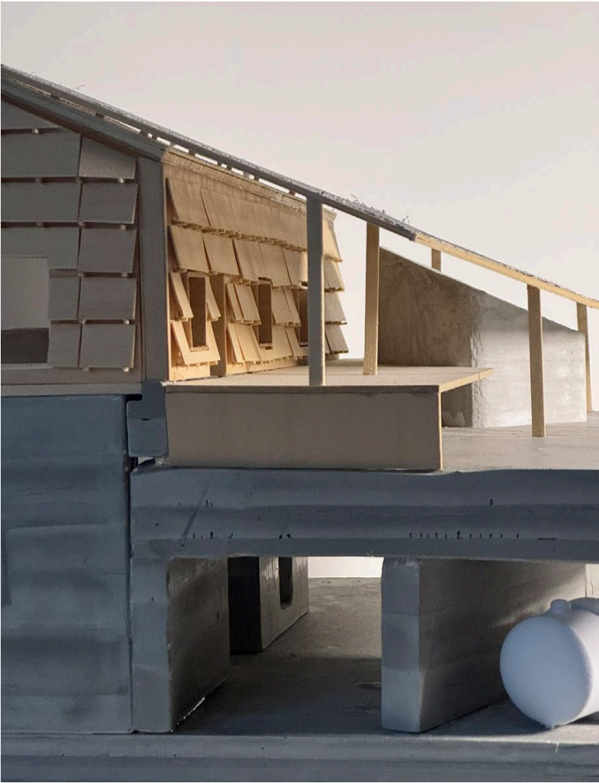
Final Model: A sectional view of the central building, showing the covered patio and factory below, complete with water storage tank.
