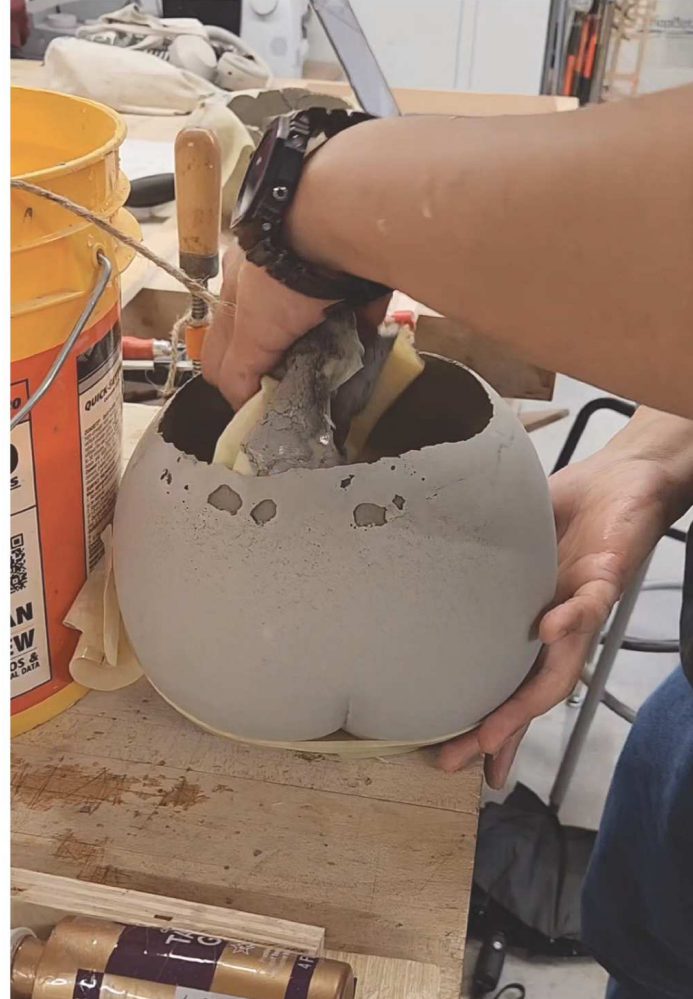
Top Left & Bottom Left & Bottom Right: Hanging Double Balloon Concrete Surface Making Process, Right: Double Balloon Concrete Surface
