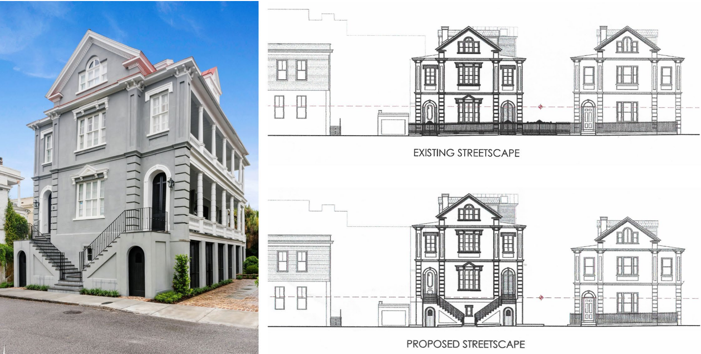
Left: Photograph of 1 Water Street Residence after elevation. Right: Streetscape change diagram for 1 Water Street, with another historic house (3 Water Street) built with the same design on its side. Source: Julia F. Martin Architects.
