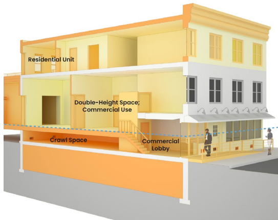
A design scheme in NYCDP’s 2014 Retrofitting report that achieved streetscape friendliness at the cost of extensive formal and structural changes, revealing the tension between Integrity & Streetscape goals.
