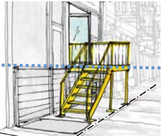
Egress stairs deployed directly over dry-floodproofing shields. Source: NYDDCP 2016, 87.
