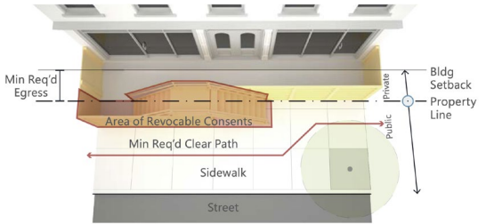
A Dry-Floodproofing Enclosure with Temporary Egress. Source: NYCDP 2014, 92.
