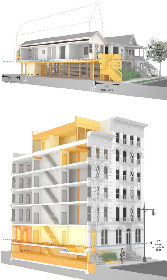
Instances of Structural Elevation and Non-Structural Elevation. Source: NYCDCP 2014, 43; 73.
