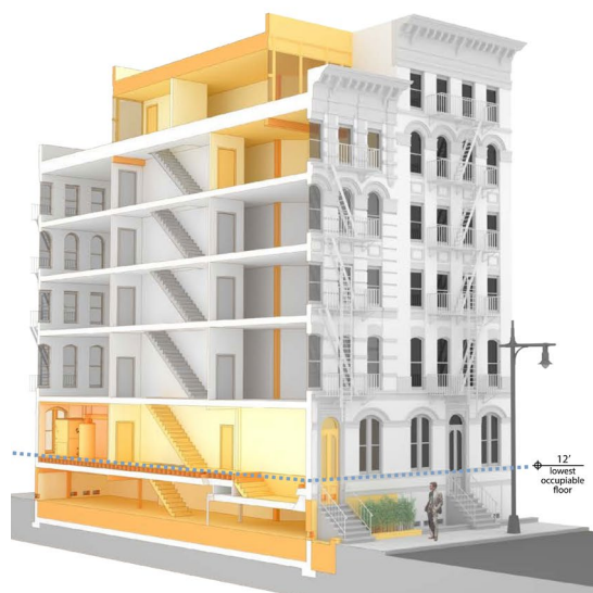
Instances of Structural Elevation and Non-Structural Elevation. Source: NYCDP 2014, 43; 73.
