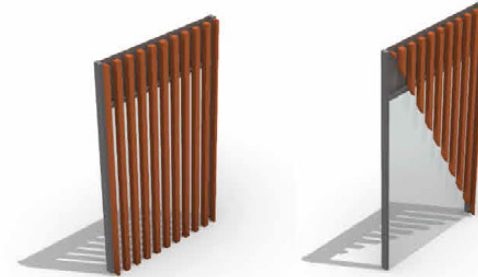
Facade Type 1: Solid Terra Cotta Unitized Panel
