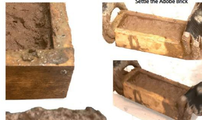
Gently Shaking the Mold Upwards to Release and Settle the Adobe Brick
