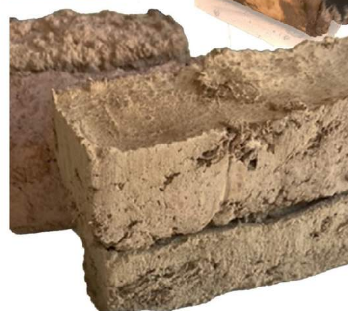
Compressing the soil within the mold, ensuring a firm and even layer. Afterward, I top it off with water to achieve a smooth, finished surface.
