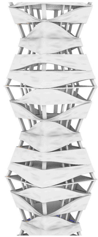
Pre-fabricated Rammed Earth Walls with Fabric formwork. Walls are formed with the combination of fabric on the front side as formwork for casting with the supports of wood formwork from remaining 3 sides. The shape after casting is bulging out, resulting in walls taking shape of fabric, which gives it an aesthetic look as well as it's properties.
