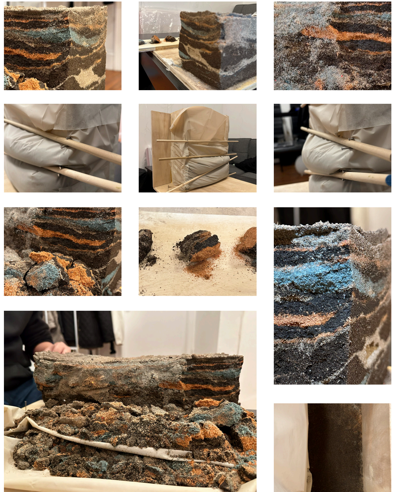
Docmentation of experimenting Rammed Earth + Fabric Formwork. Formwork was created with three wooden planks and a fabric supported by some sticks in front. The purpose of stick was to give wall a shape after ramming earth into this formwork. One by one, each layer of earth with different compositions were rammed.
