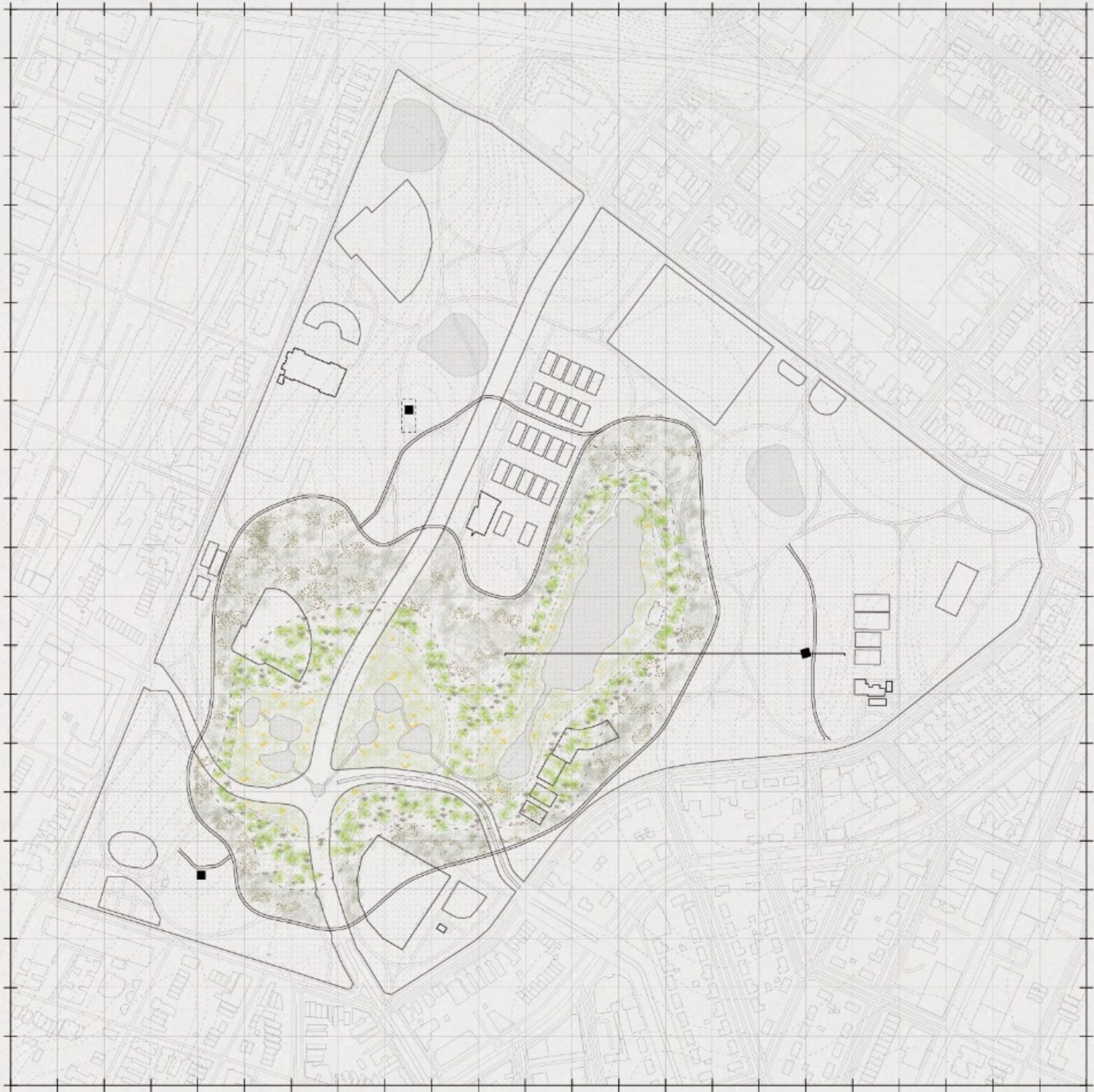
Large Infrastructure Plan (Extreme Response) During extreme flooding scenarios, stormwater is redirected via the canal system into low lying areas in the park delineated by flood tolerant landscaping. A new masterplan for the park driven by this floodplan is overlaid and water monitoring stations replace existing social spaces in the park as a way to educate the public about issues surrounding living with water in the city.
