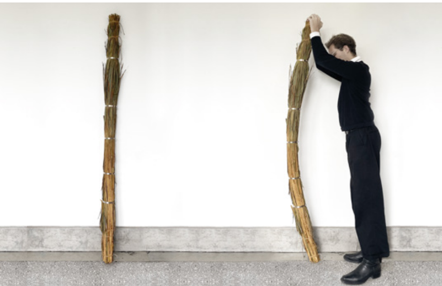
Structural test of reed column, not suitable parallel to load
