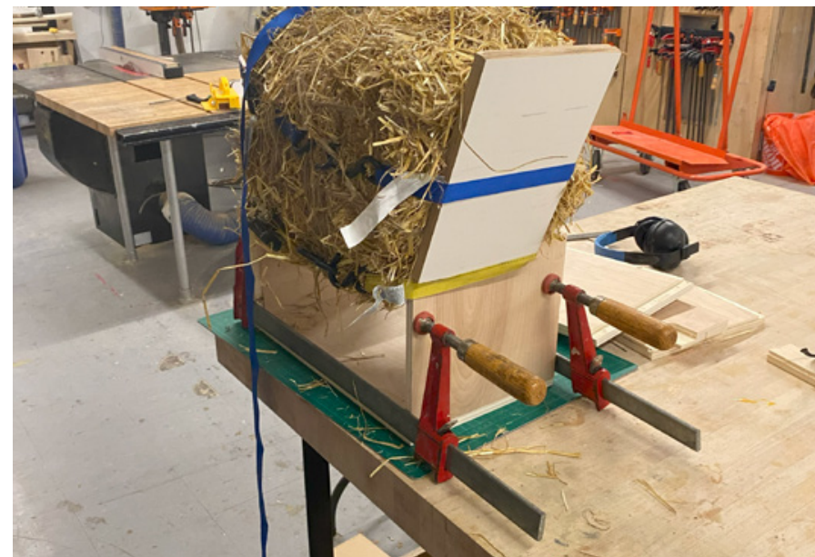
Compressing the straw to ensure structural integrity
