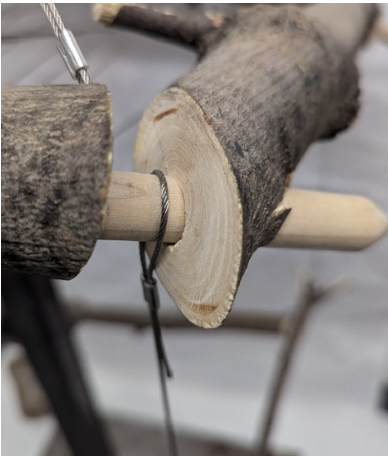
Dowel detail through a miter
