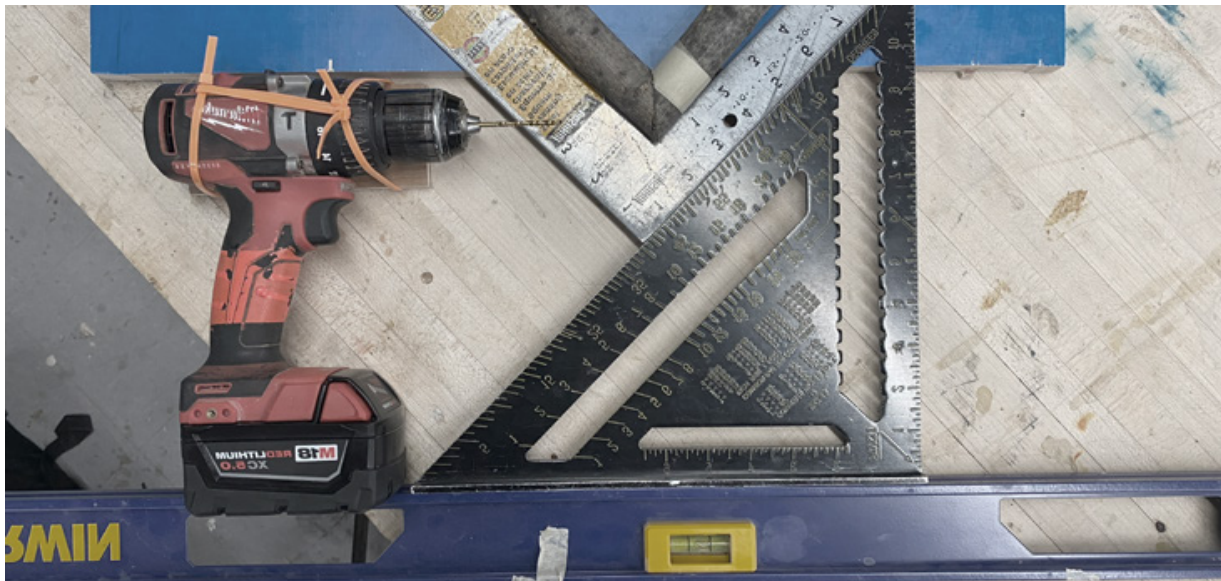
Numerous jigs were used to ensure that all of the holes were straight and even
