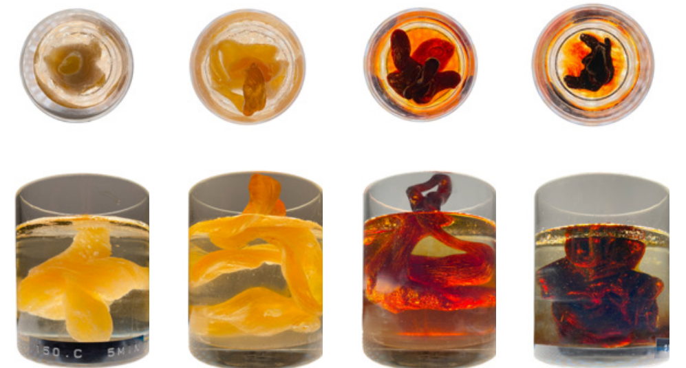
Sugar is melted and pulled at different temperatures corresponding to molecular change
