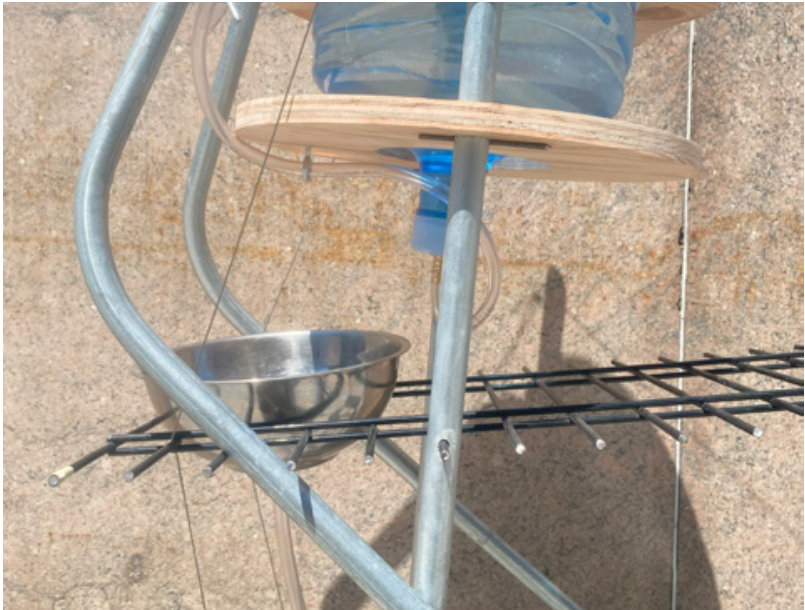
Horizontal elements slot into holes in the vertical element
