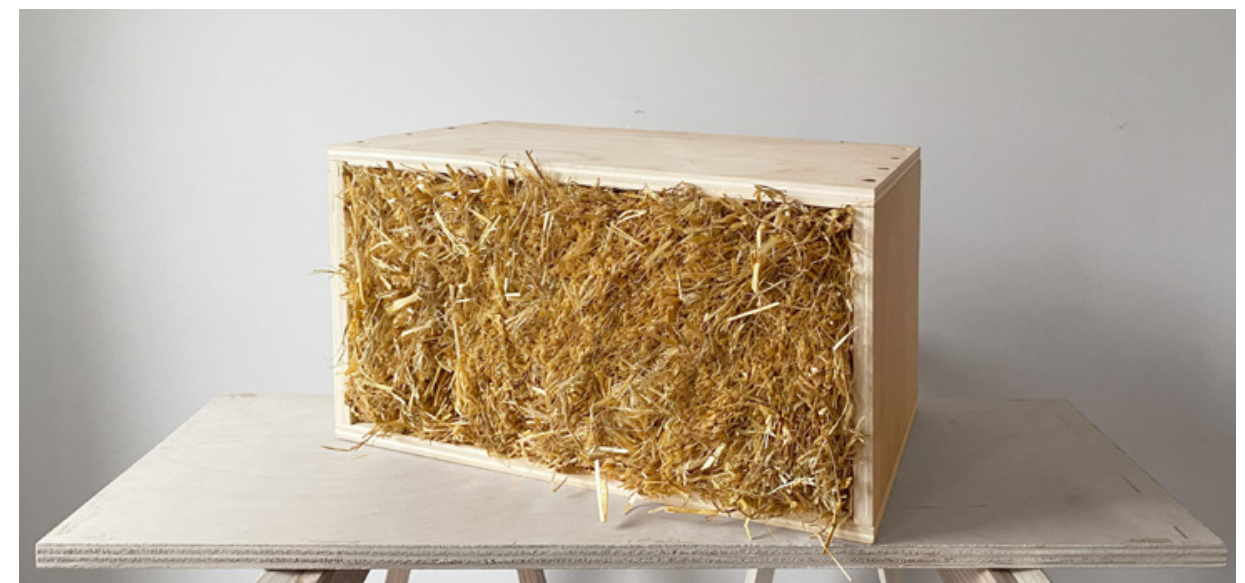
Structural straw block mock up, grasses strongest when compacted and load perpendicular to stalk
