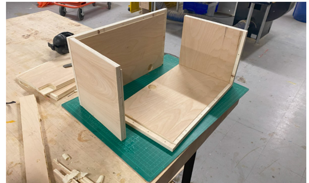
Structural plywood frame to contain and load the straw
