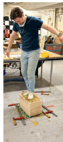
Compressing the straw to ensure structural integrity
