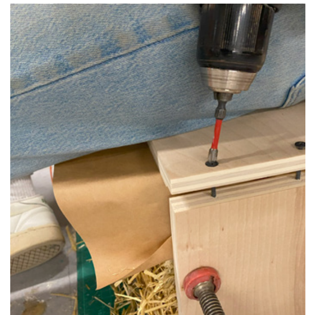
Structural plywood frame to contain and load the straw
