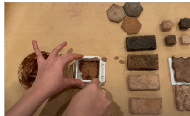
SLURRY POURED INTO MOULDS
