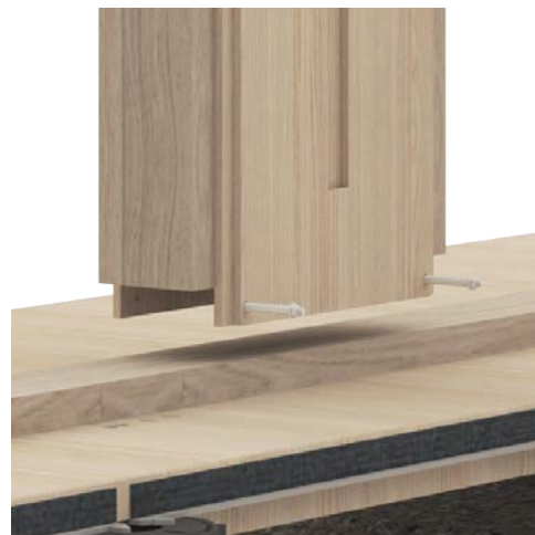
Wall panel mounting over guide rail
