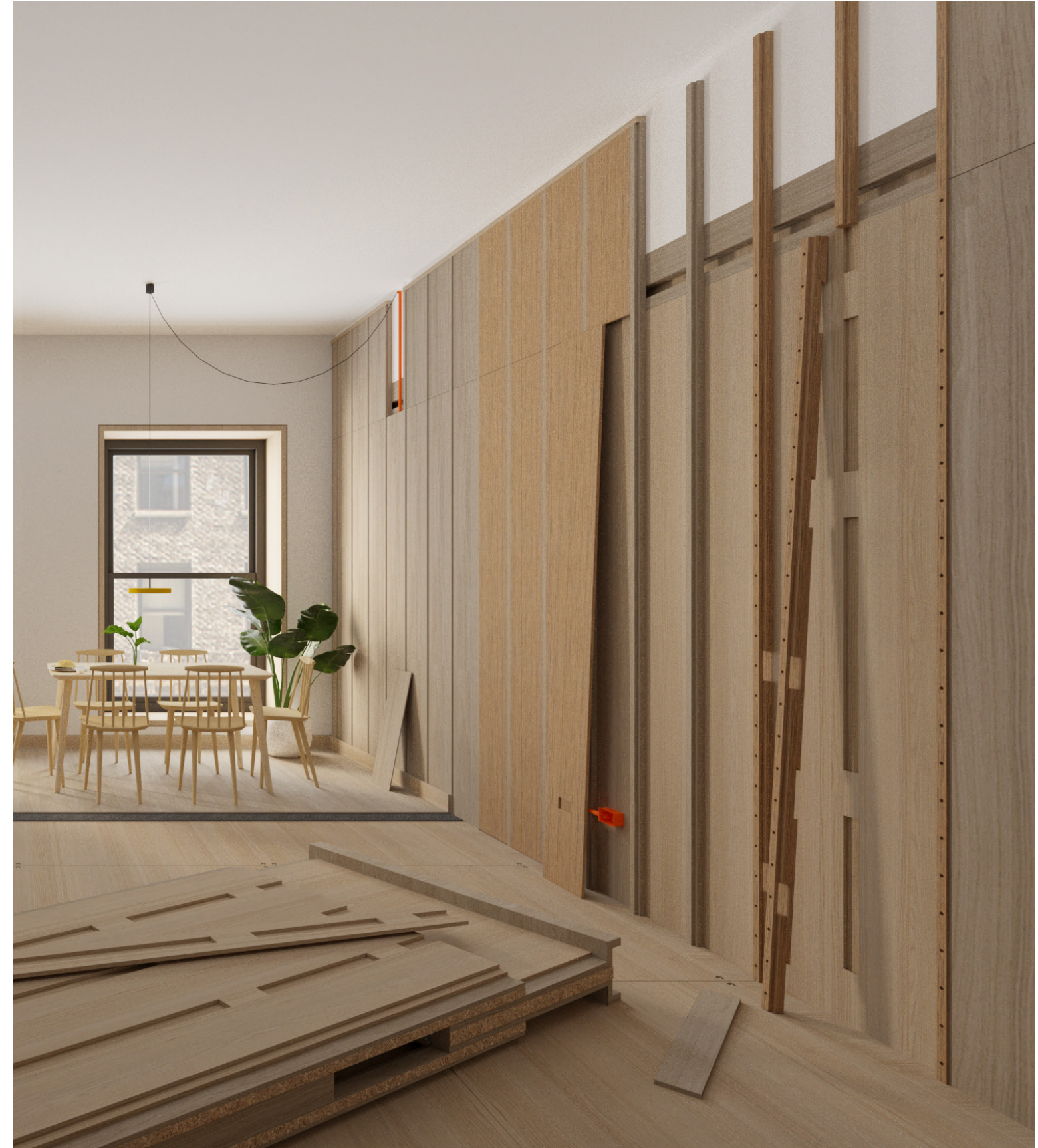
Mounting and assembly system
