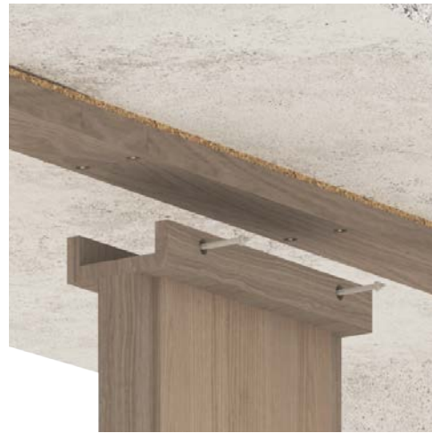
Attachment of wall panel to guide rail
