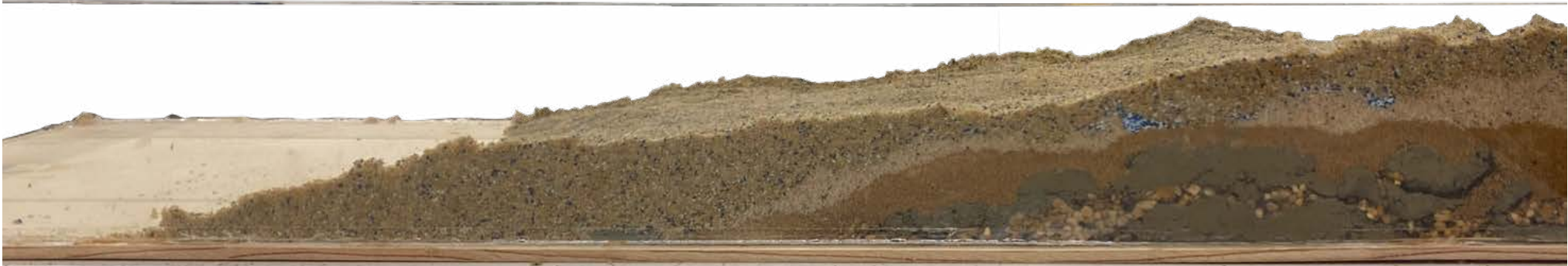
RIVER SIMULATION MODEL | Acrylic sheet, plywood, various sand grains of different colors to help visualize sediment movement.
