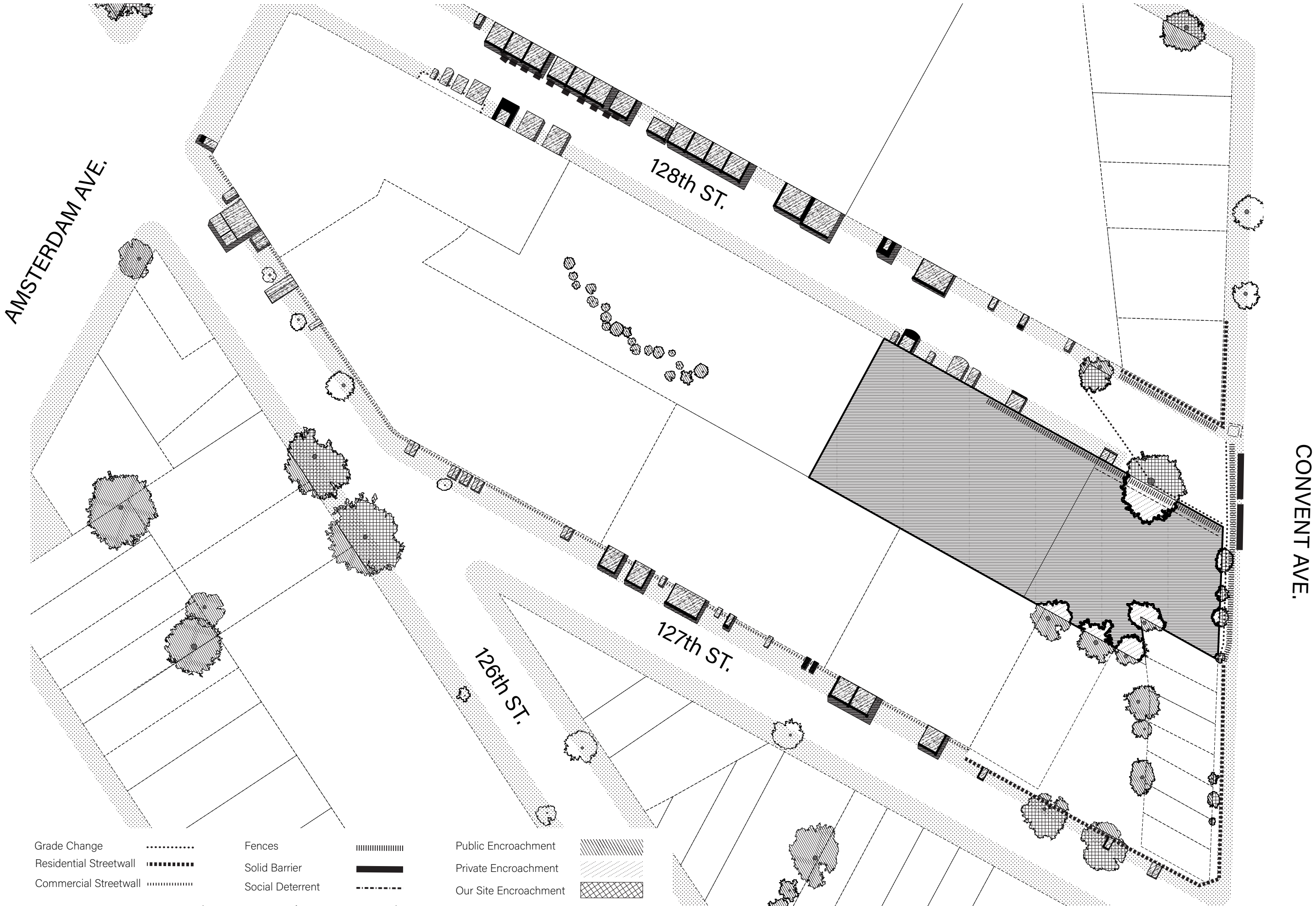
SITE ANALYSIS / Mapping social and physical barriers and encroachments, with particular focus on industrial scale doorways and openings
