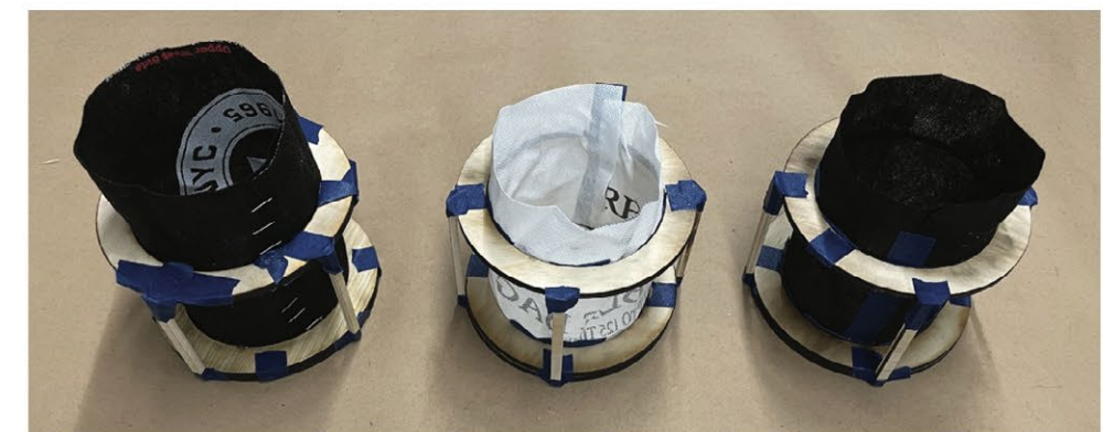
Building the formwork with fabric and a scaffolded structure around it.
