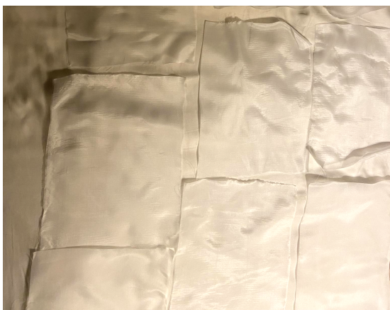
The silk sheets after being printed with UV ink, shown under incandescent lighting.
