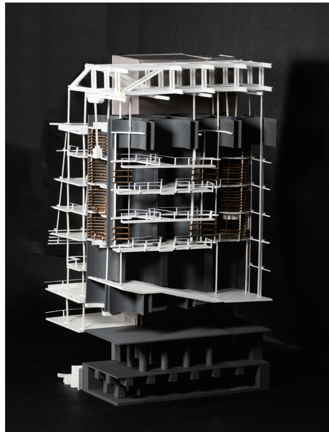
Chunck Model: Reinforce the existing vertical circulation and some silo structures to serve as the main supporting structure for the hanging system.
