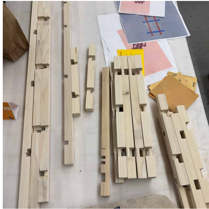
RIGHT ANGLE CUTS WERE COMPLETED ON THE TABLE SAW
