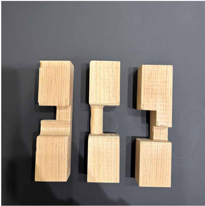
3 TYPES OF CUTS FORM THE JOINT
