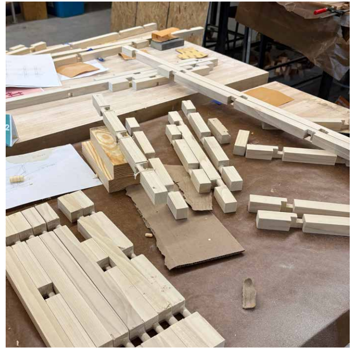
PIECES WERE SANDED DOWN FOR TOLERANCE CONSISTANCY
