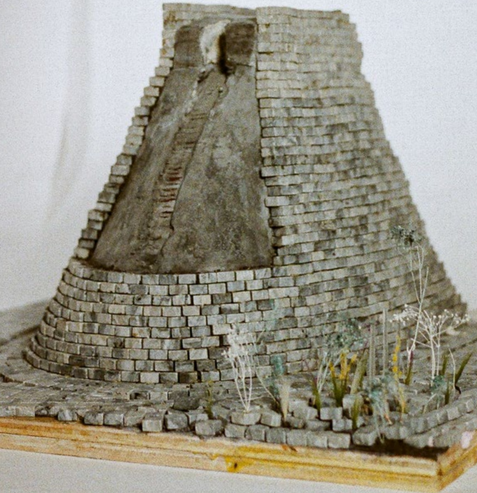
Model of the vault structure in stone.
