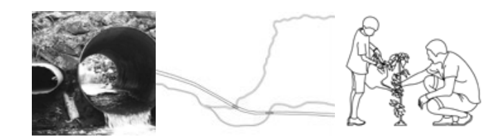
ECOLOGICAL DAMAGE: ROAD CREEK CROSSING replace the culvert with bridge; plant seedling on the eroded ground at the triangular area of the road-creek crossing
