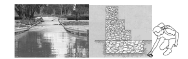
ECOLOGICAL DAMAGE: FLOOD put rock into the gabion wall as foundation at the sharp turn of the creek to mitigate the flood
