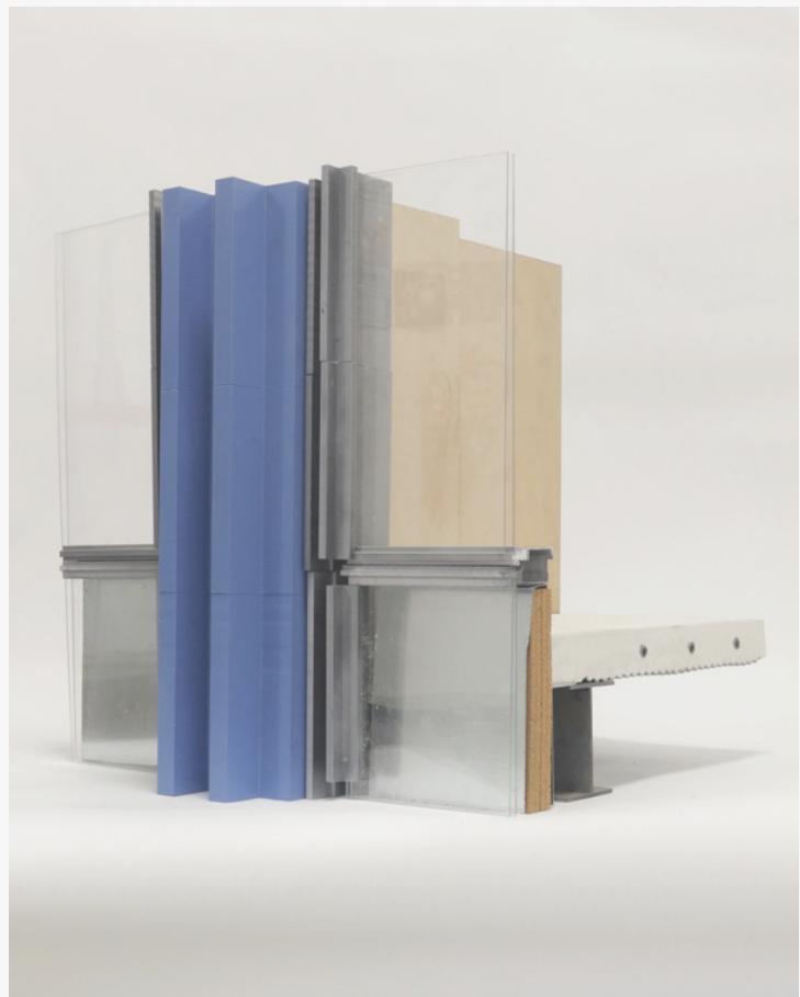
unitized curtain wall and custom column cap 1" = 1/4" physical model with construction drawing set with Ian Callender and Gio Kim
