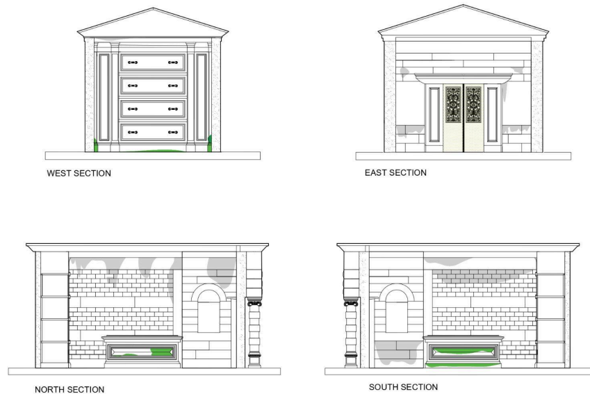
Figure 7 Mausoleum Interior Condition Drawings
