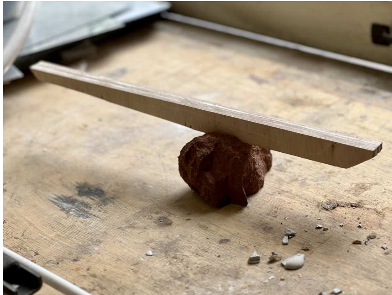
Roughness of the stone carved into the refined geometry : using stone's irregularities to provide compressive strength to cantilevering refinements.
