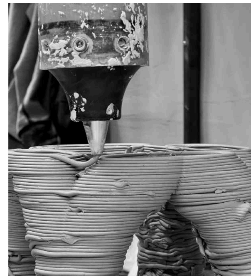
▼ Component C : 3D printed sawdust - facade components - Evaporative-Cooling Screen
