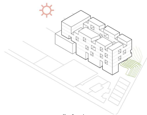
Perforation Openings improve cross ventilation, increase day-lighting, and foster vibrant communal spaces
