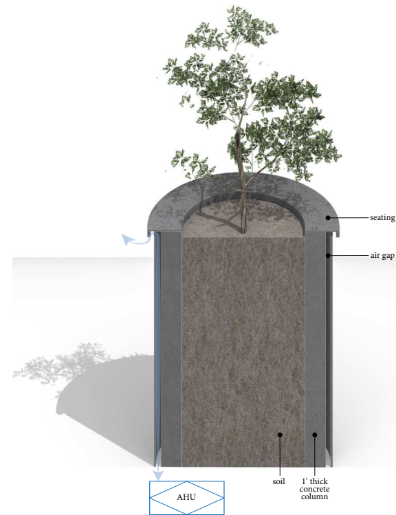
Planter Ventilation Detail
