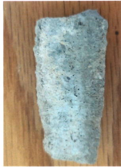
Figure 9 Repaired Mortar, Photographed by W. Sun.
