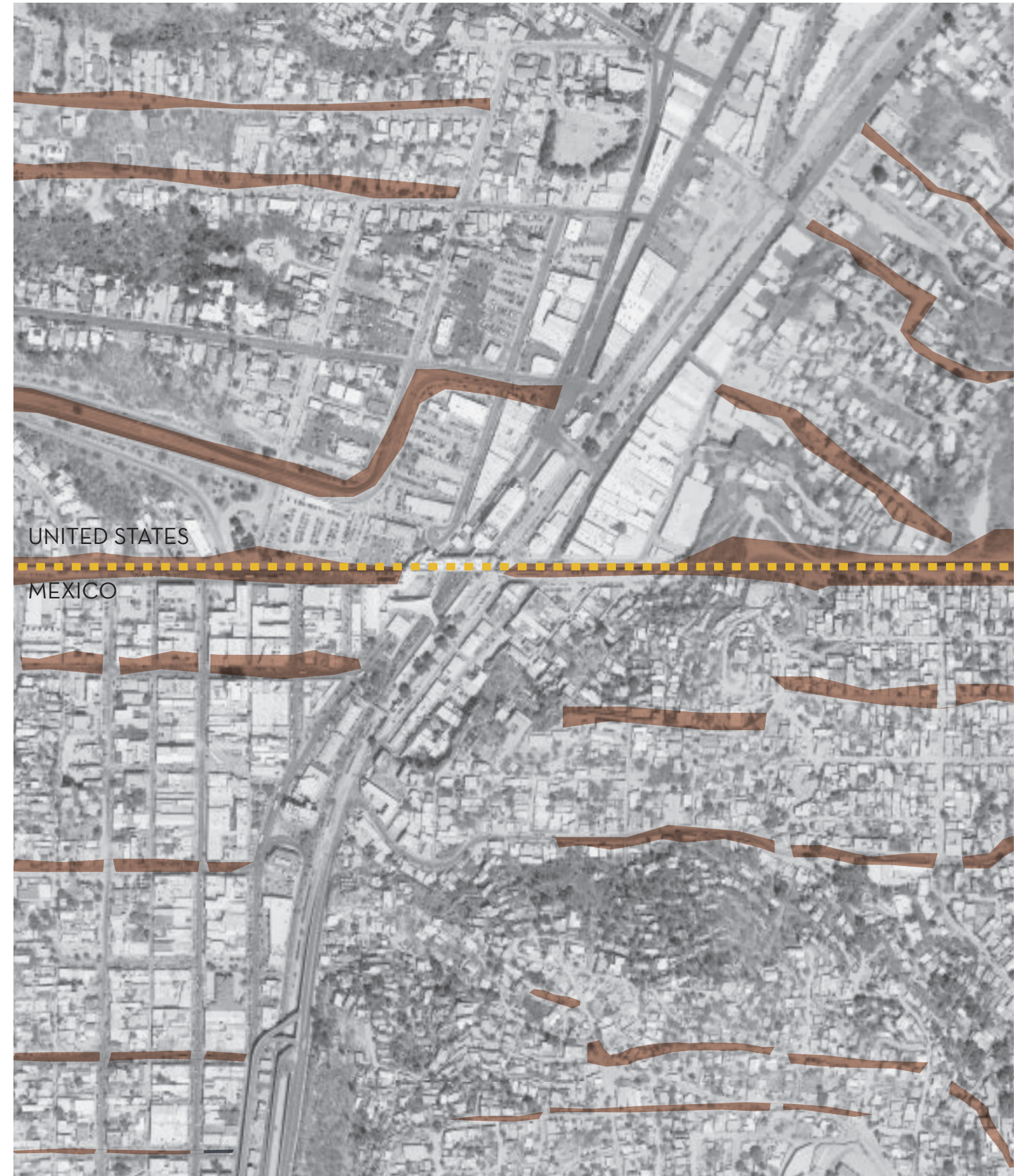
Dismantling the border wall and implementing bioswales are the first steps in this proposal to address the issue of flooding in Ambos Nogales. Bioswales will work in conjunction with an updated storm water drainage system to assist with storm water runoff. 7 The proposal includes bioswales of varying sizes, the largest of which is located at the border site and subsequent ones reducing in size as they move further from the central axis.
