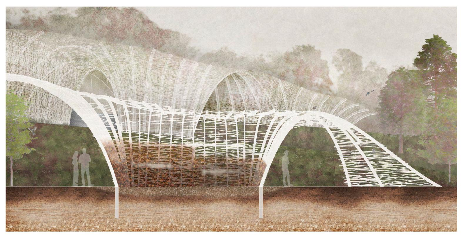
(above) detailed section through a terramation node woven with branches in a wattle construction method with CLT primary members
