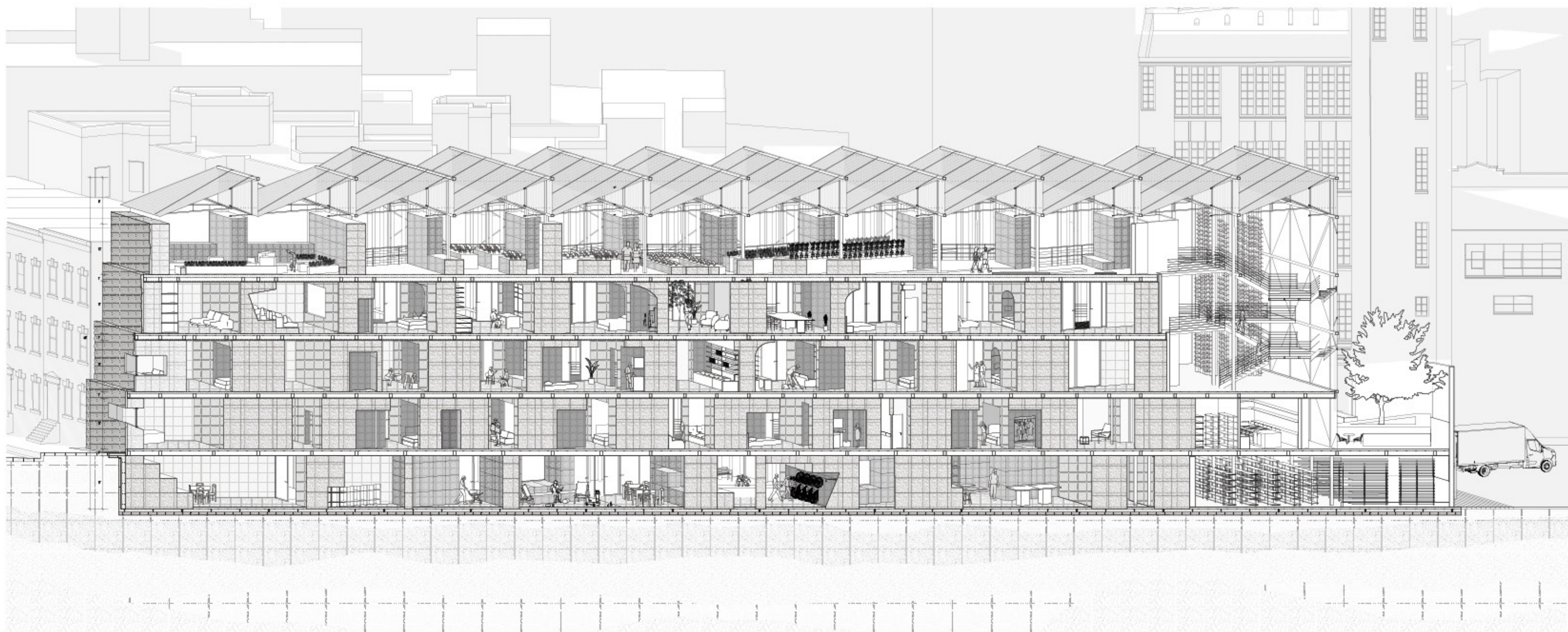
Large straw bales serve as the modular building blocks for the construction logic. Starting as full coverage at the ground floor, less straw is needed as you go up the building allowing for the bales to recede. The massive walls are an opportunity for space. When walls are massive, space is carved from the mass. As you ascend the building, space is held between walls. Inhabitation transitions from bottom to top following the logics of mass straw bale construction.
