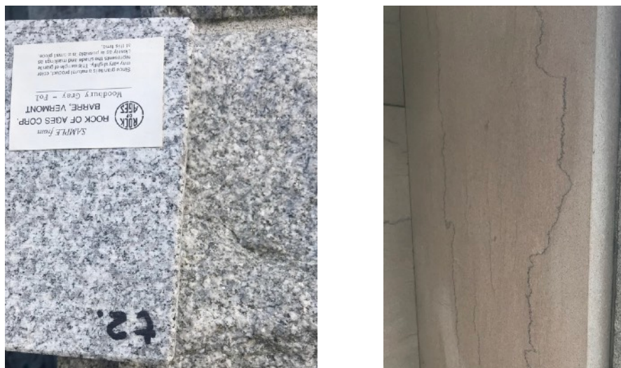
Fig. 9 (left): Comparison of Barre granite sample and mausoleum. Fig. 10: Polished limestone interior.
