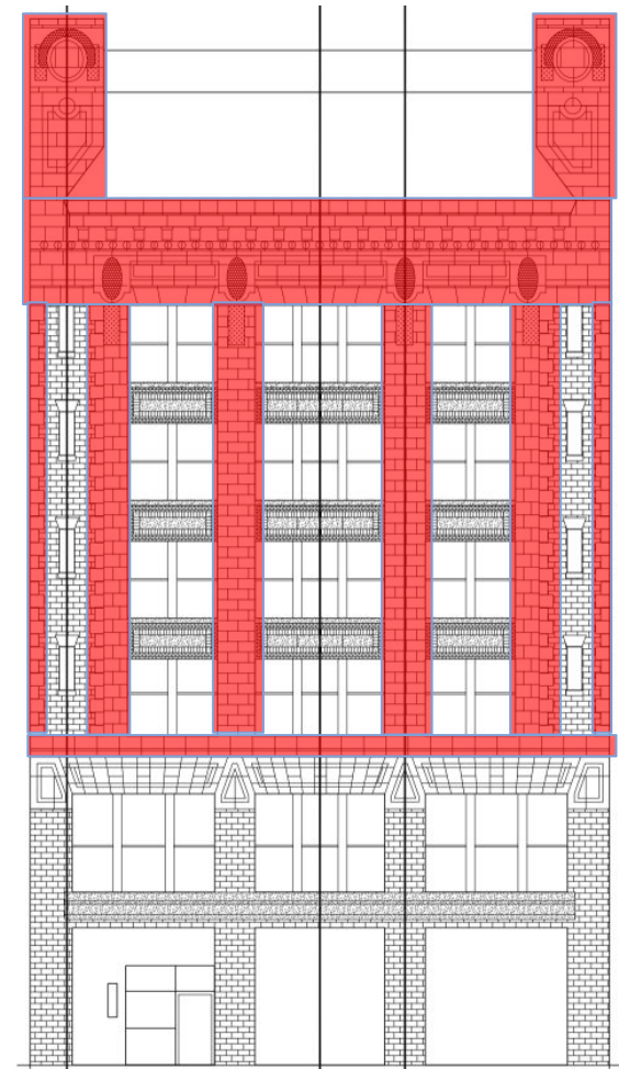
TERRACOTTA ON FACADE Sheffield Farms by Columbia University
