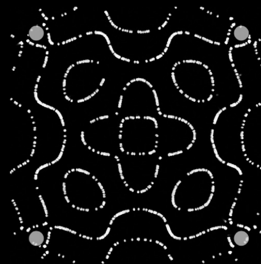
ELEVATOR SHAFT 352 Hz / -90.6 dB
