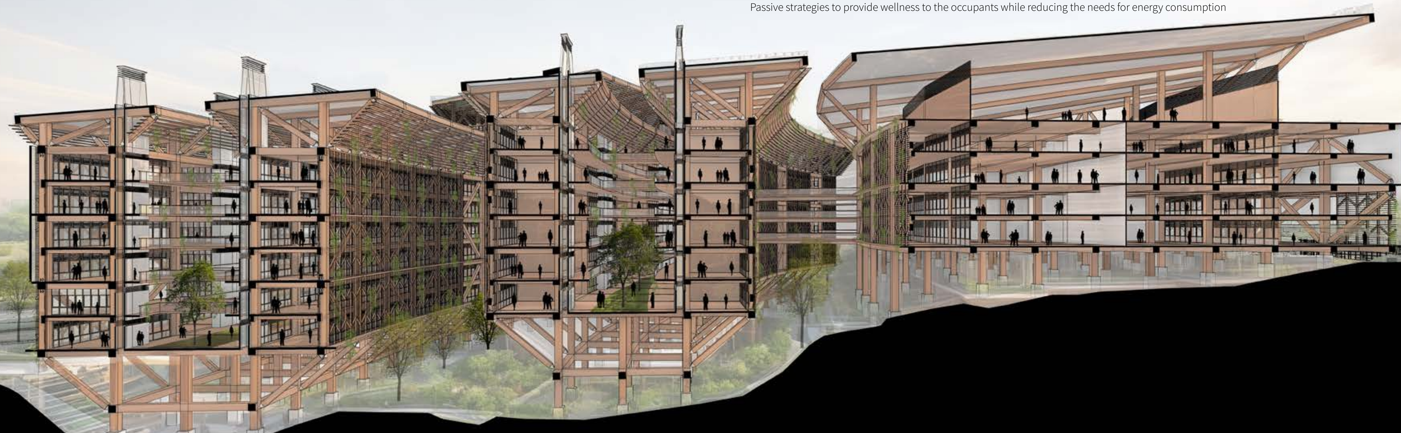
Overall section of the Legislative Building Complex, showing atriums inside and gaps between buildings, and the stilt concept as a response to the hilly land site
