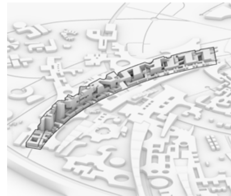
Cut and interlock the mass, introduce openings toward NW-SE axis and in podiums
