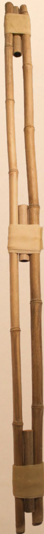
BAMBOO + RUBBER JOINT: DETAIL SCALE 1:1
