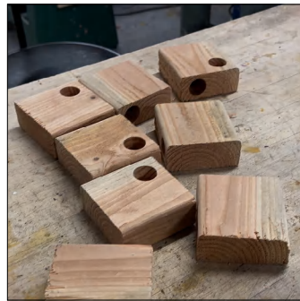
Make 8 joints, with 3 holes on each of them.
