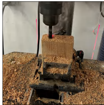
Make 8 joints, with 3 holes on each of them.
