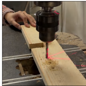
Cut four boards, slote them so they can spell together. Then punch holes on each board.
