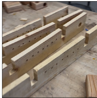
Cut four boards, slote them so they can spell together. Then punch holes on each board.
