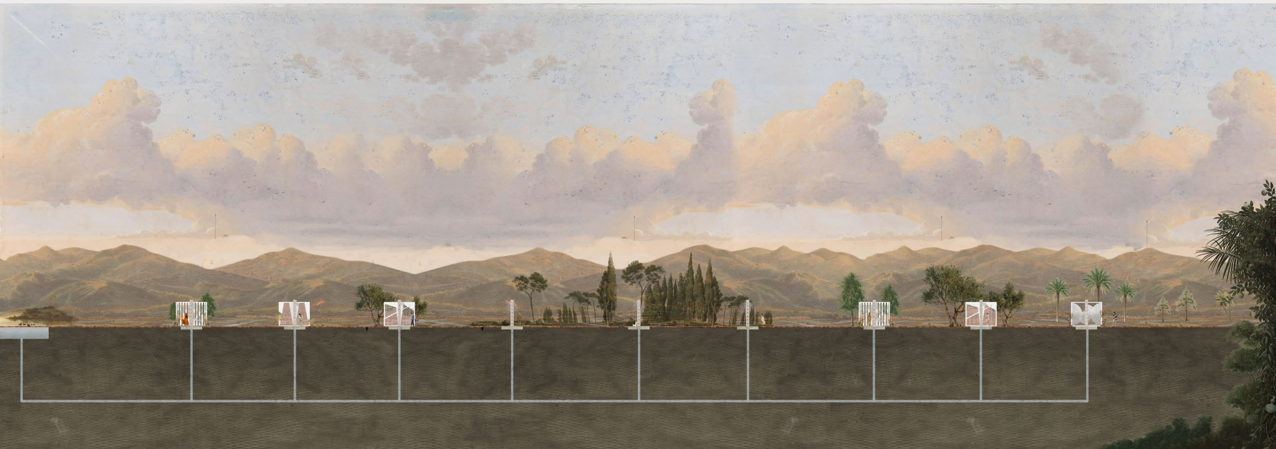
Section cut showing the use of water from the bi-communal water treatment plant in the Green Line to supply misting units at each portable station during the hot summer months.
