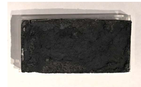
30% ground biochar 70% pre-mixed concrete more water
