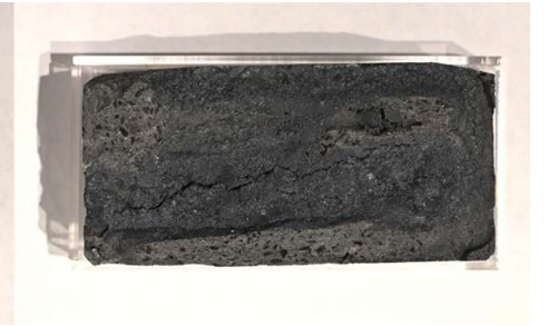
10% ground biochar 90% pre-mixed concrete
