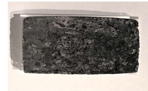
20% not ground biochar 80% pre-mixed concrete
