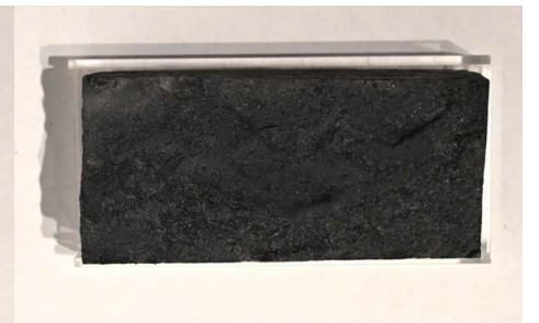
20% ground biochar 80% pre-mixed concrete
