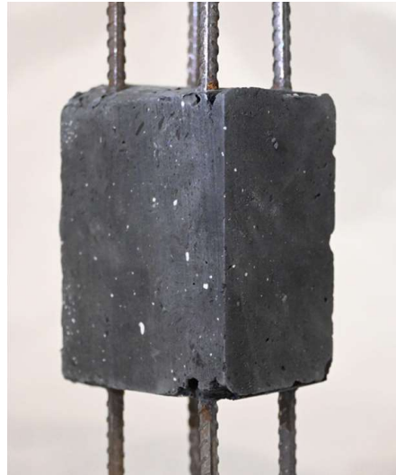
30% ground biochar 70% portland cement 0.00502kg C/kg
