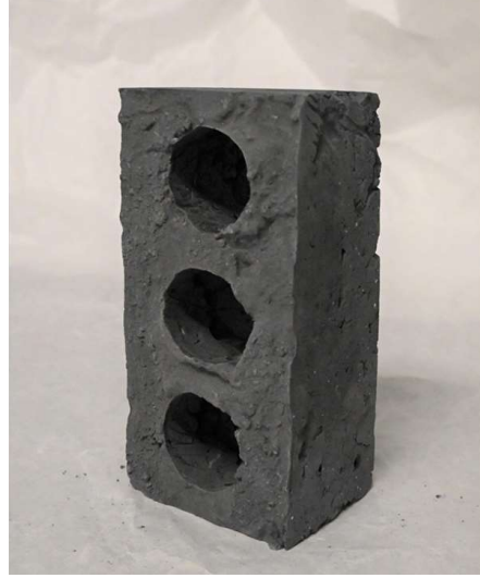
30% ground biochar 70% portland cement 0.00502kg C/kg
