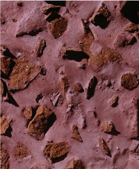
Material Experiment Waste Brick, Cement, and Pigment as a New Wall Technique
