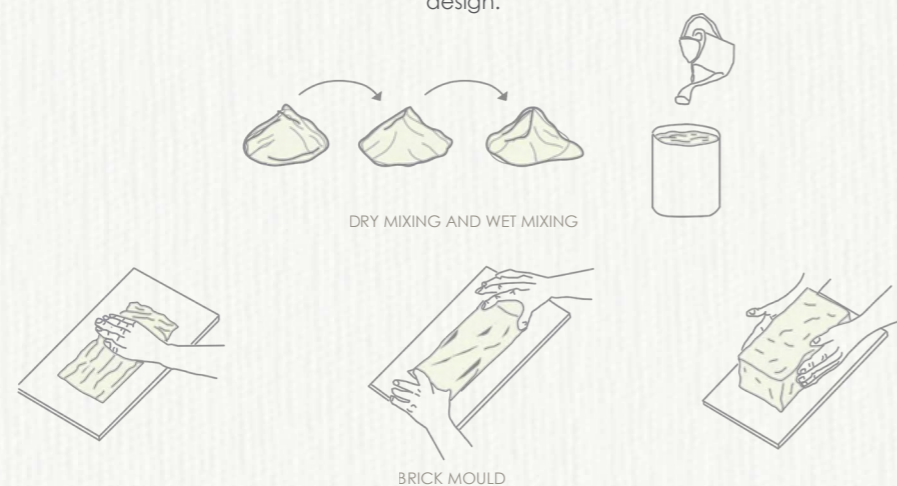
Sugarcrete Block production
