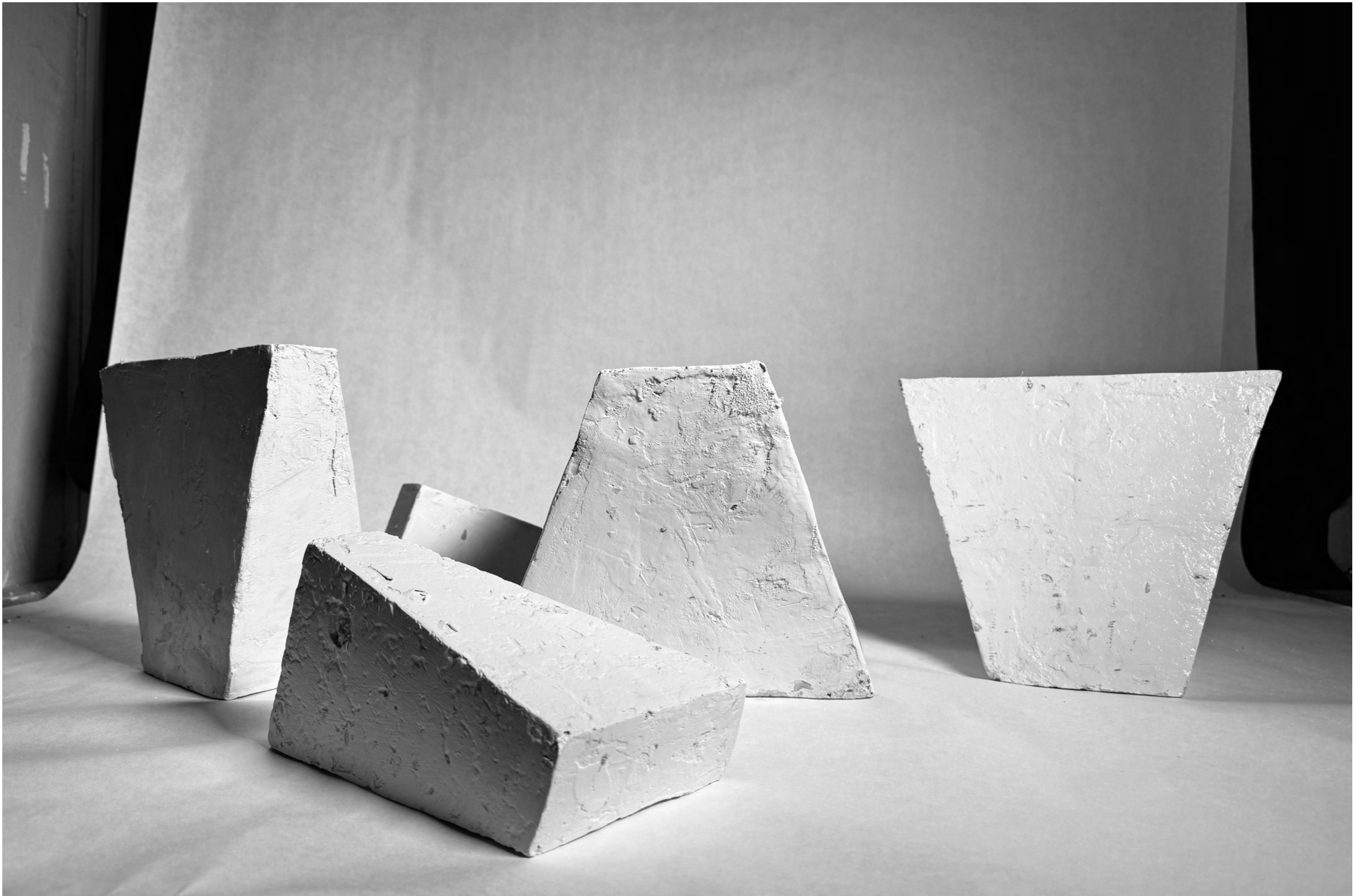
1:1 Sugarcrete blocks (bagasse +Lime)
