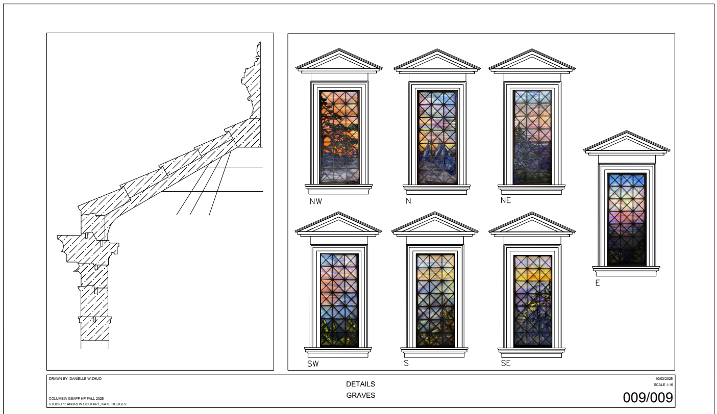
Figure 14: Details of mortise and tenon roofing system (left) and 7 impressionist Tiffany & Co. stained glass windows (right) in Graves Mausoleum
